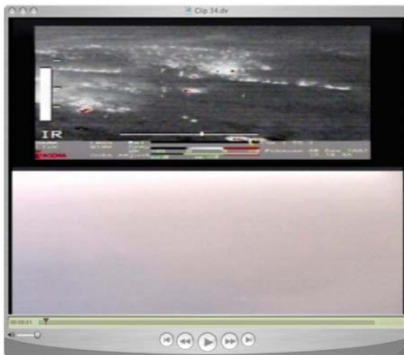
Fig. 6 This image taken 5 Dec 2002 near Borowra shows the difference FLIR can make to critical intelligence collection. (Top image is TIR and bottom image is the visual bands). Without FLIR the bottom view is all the crew can see
